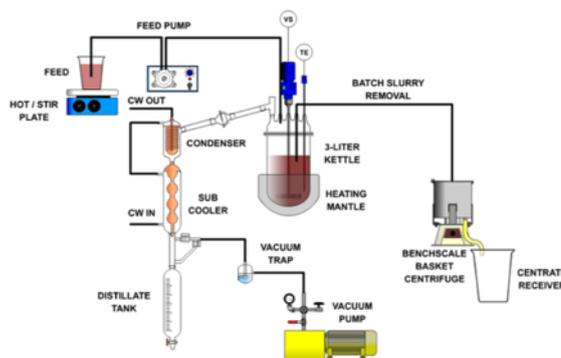
Figure 3. Schematic crystallisation bulk test programme flowsheet design.
