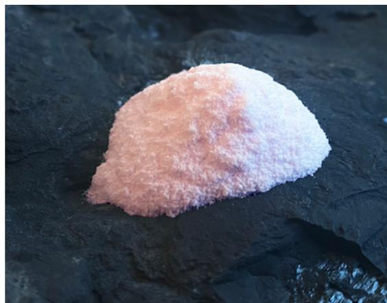
Figure 5. Element 25 HPMSM crystalline product.
