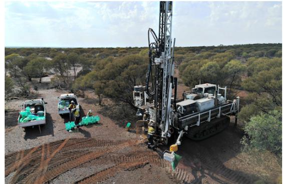
Figure 5: X350 track mounted aircore drilling rig.
