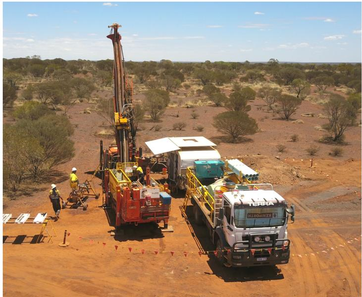
Figure 3: Diamond Drilling at Butcherbird February 2019.
