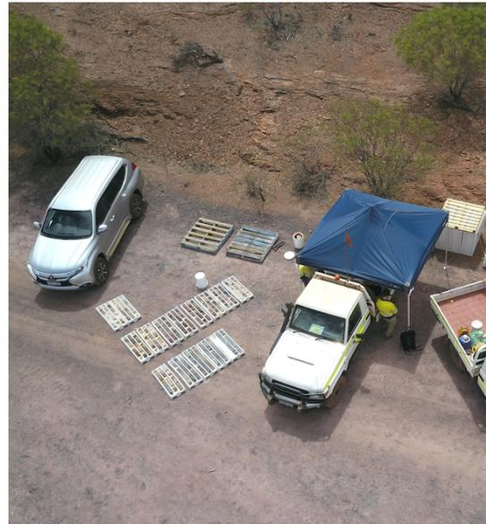
Figure 2: Drill core laid out for logging.
