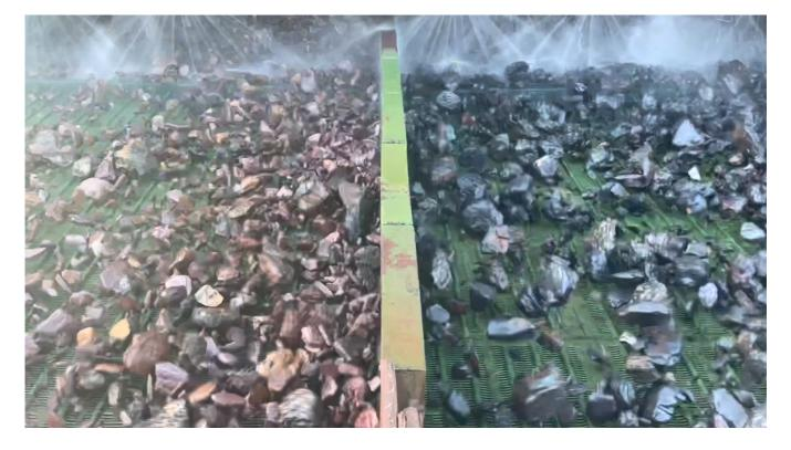
Figure 2. Butcherbird feed material on the wash screen after densimetric separation showing a clear delineation product and waste.
