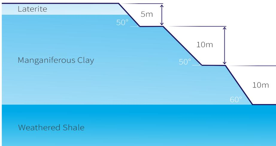
Figure 3: Yanneri Ridge – Limit Equilibrium Analysis Model and Proposed Pit Parameter
