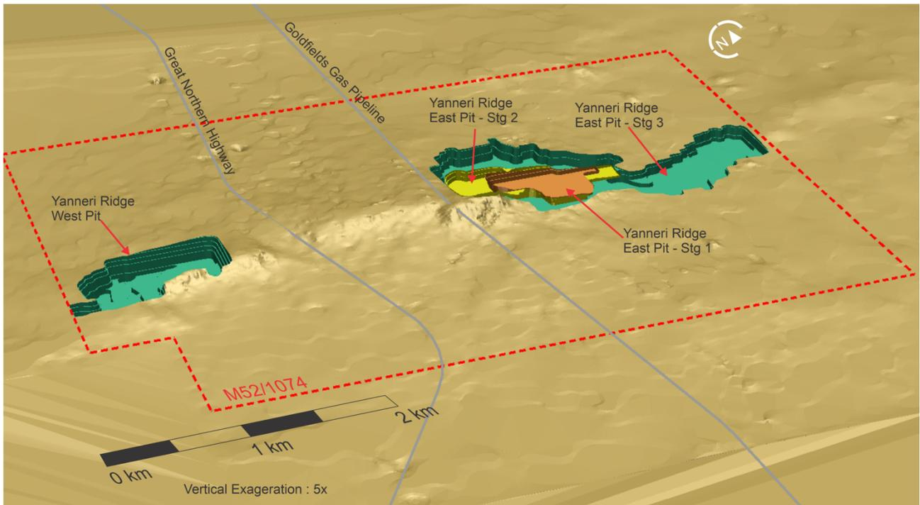
Figure 1: Pit designs (Isometric view looking North East) for the Yanneri Ridge deposit showing open pit staging
