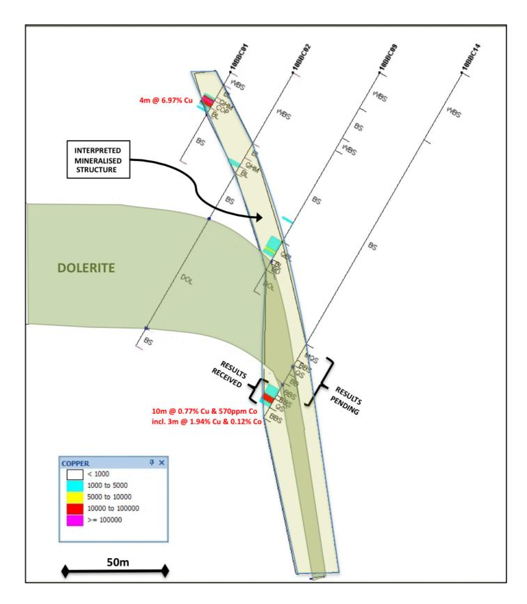
**Figure 1:** Schematic cross section through copper mineralised zone at the Butcherbird Copper Prospect showing the relationship between the dolerite intrusive and interpreted mineralised shear system.
