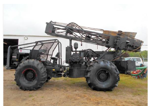
Figure 2: Soil test borehole drilling rig.
