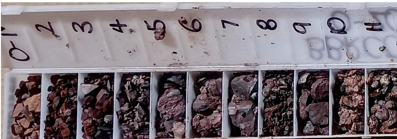
**Figure (1.3.3): Lateritic manganese mineralisation intercepted in exploration drilling at the Butcherbird Project**
