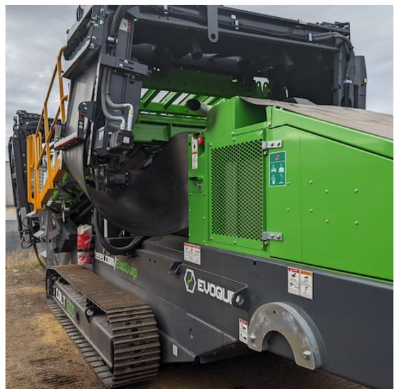
Figure 2. Scalper being prepared for mobilisation.
