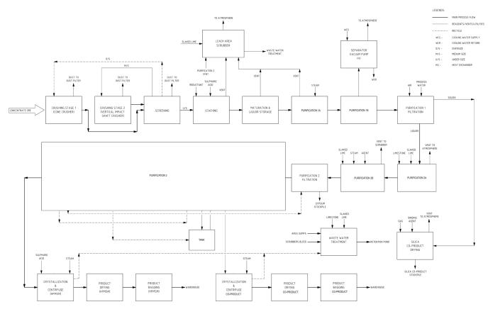
Figure 3: Schematic outline of the E25 HPMSM Process.
