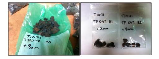
Figure 1. Screened +8mm material and assay samples selected from Bindi Bindi Hill screening test work.
