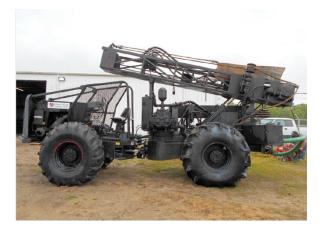
Figure 2: Soil test borehole drilling rig.
