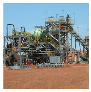
Figure 11. Bootu Creek DMS processing plant (ref: DRA Global)
