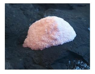
Figure 5. Element 25 HPMSM crystalline product.
