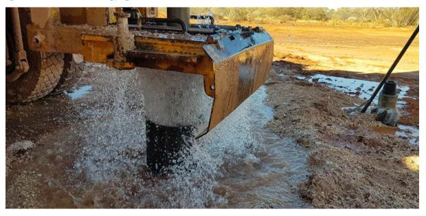
Figure 2: Pump Testing equipment set up to test aquifer yield potential.
