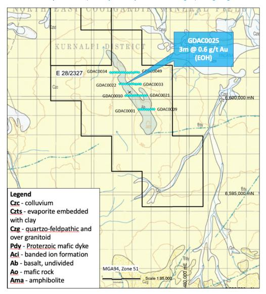
Figure 8: Green Dam aircore drilling programme collar location plan over surface geology.
