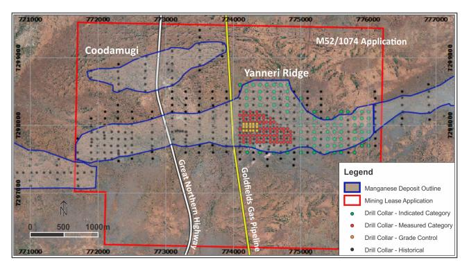
Figure 6: Completed infill drilling collar locations in relation to the previous drilling, Yanneri Ridge and Coodamudgi resource outlines and infrastructure.
