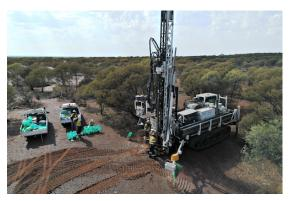
Figure 5: X350 track mounted aircore drilling rig.
