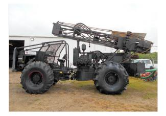
Figure 2: Soil test borehole drilling rig.
