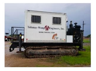
Figure 1: Cone penetration test (CPT) track mounted rig.
