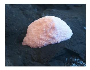
Figure 4. Element 25 HPMSM crystalline product.
