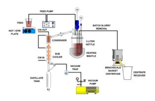
Figure 2. Schematic crystallisation bulk test programme flowsheet design.
