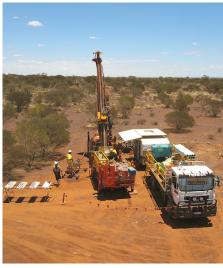
Figure 1: Diamond Drill Rig.
