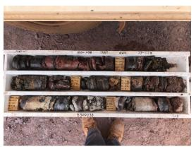
Figure 3: Manganese bands within weathered clays.
