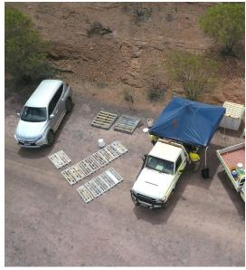
Figure 2: Drill core laid out for logging.
