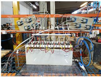
Figure 2: Electrowinning test rig at Simulus Laboratories.
