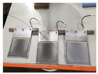
Figure 3: High Purity EMM plated onto the cathodes.
